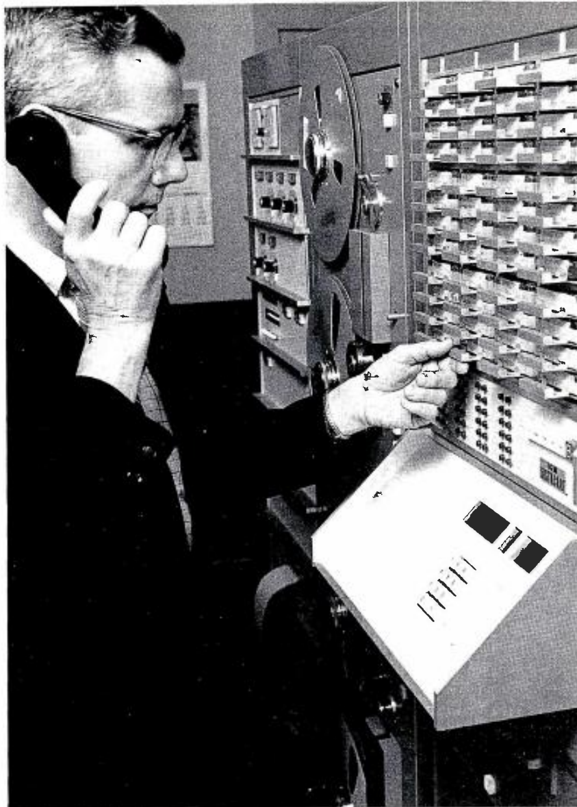
Above, general manager Morgan with WTTR's IGM 500 equipment, including 10-step music sequencer, network switcher, automatic logger with verified printout, time announcer, Instacart, and MOS memory.
